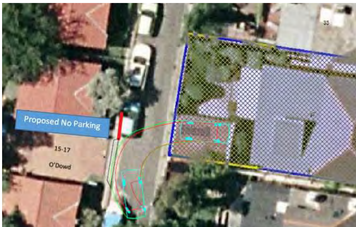
Figure 2. Swept wheel path of B-85 Vehicle and proposed NO PARKING zone
