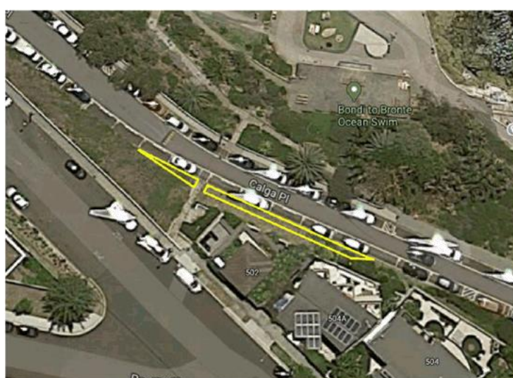
Figure 2. Widening required for Option 1B.
