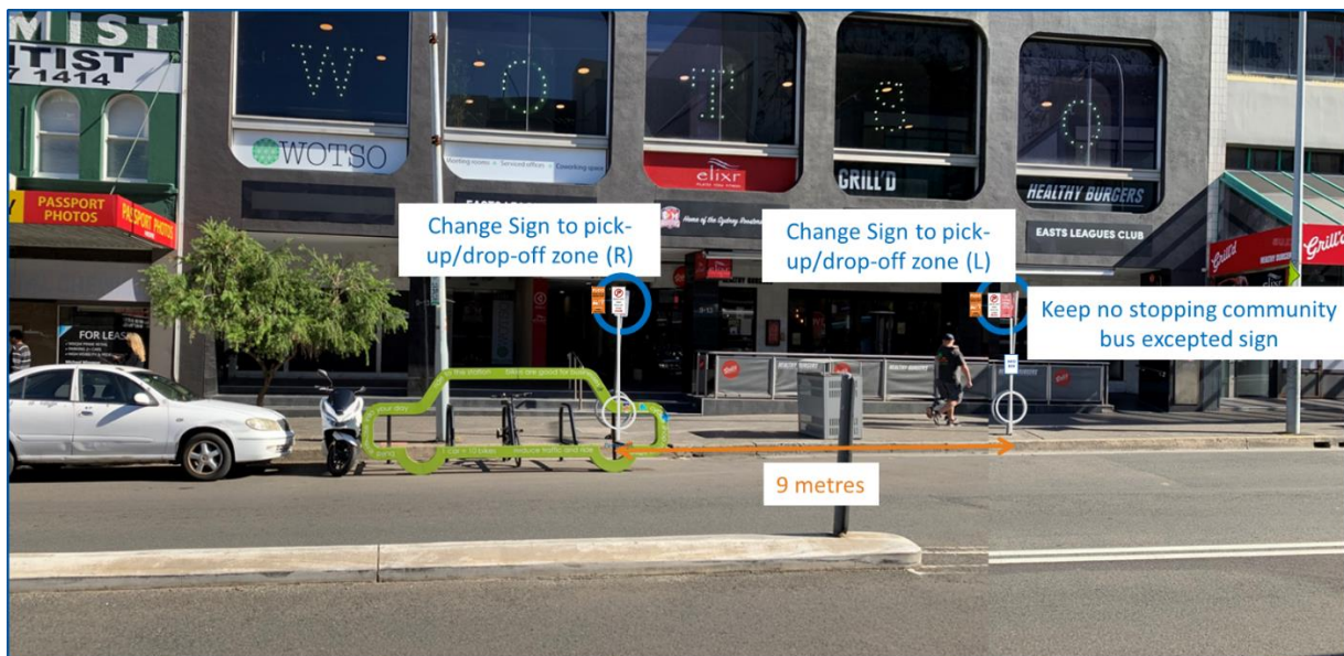
Figure 3. Proposed 9 metre PUDO bay to be operational until cycleway works are complete.
