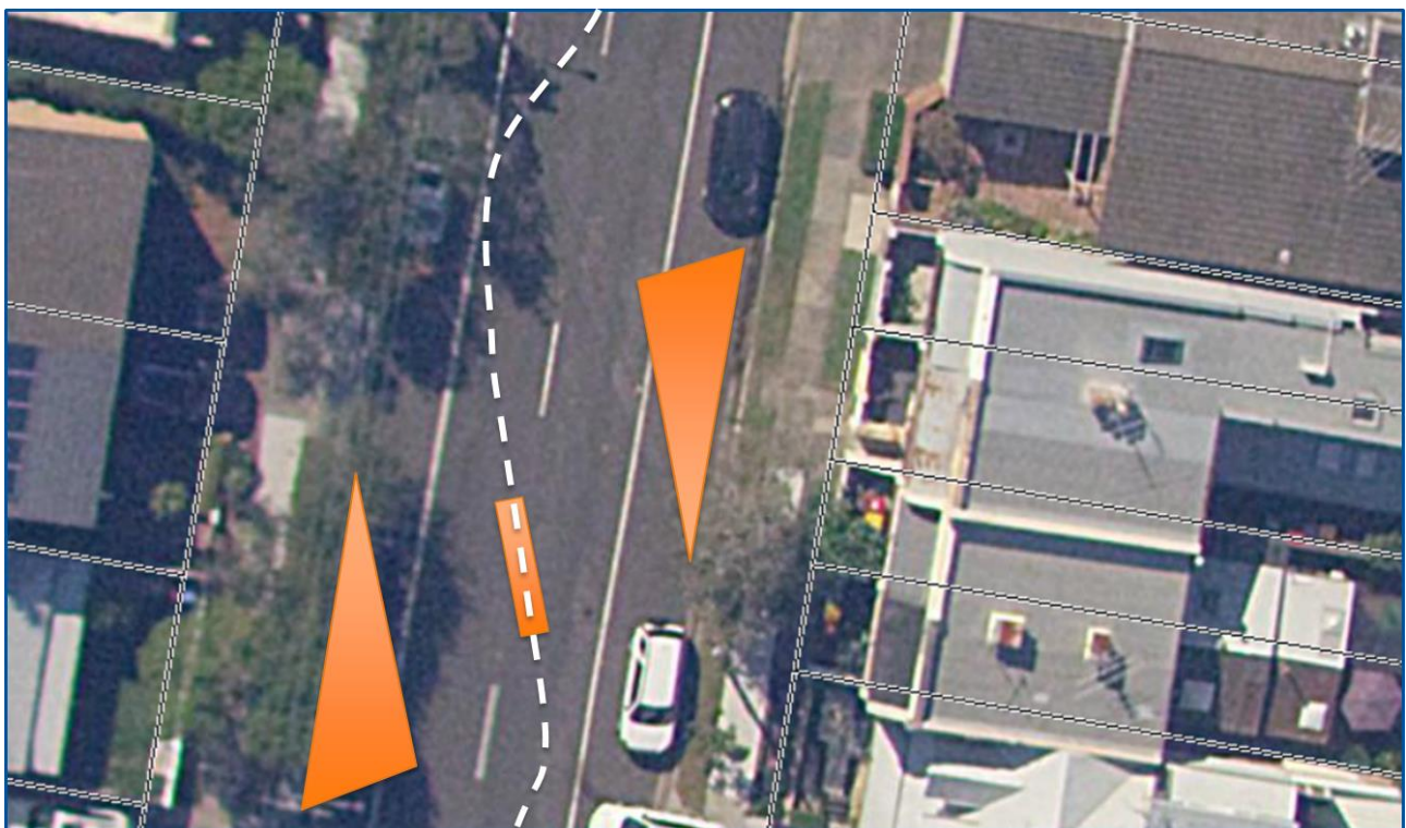
Figure 5. Option 1 – Two-lane slow point (chicane).
