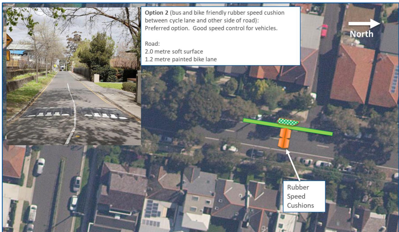
Figure 6. Option 2 – Rubber speed cushions with a reduced kerb island width to allow for a 1.2 metre bicycle plus green painted bicycle marking (recommended option).
