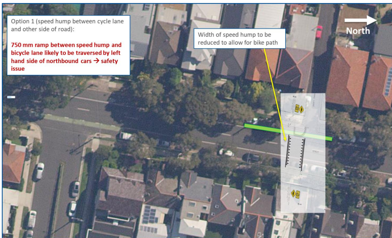
Figure 5. Option 1 – Original design with a reduced kerb island width to allow for a 1.2 metre bicycle lane plus green painted bicycle marking
