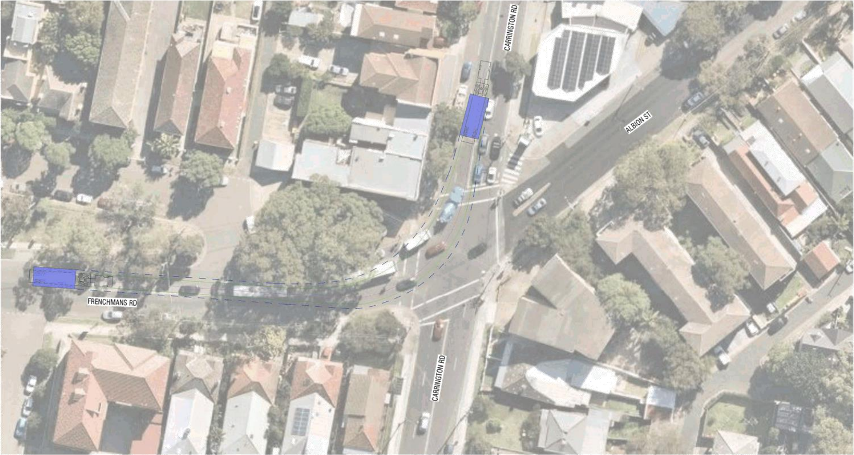
Frenchmans Rd Turning Left into Carrington Rd Swept Path
