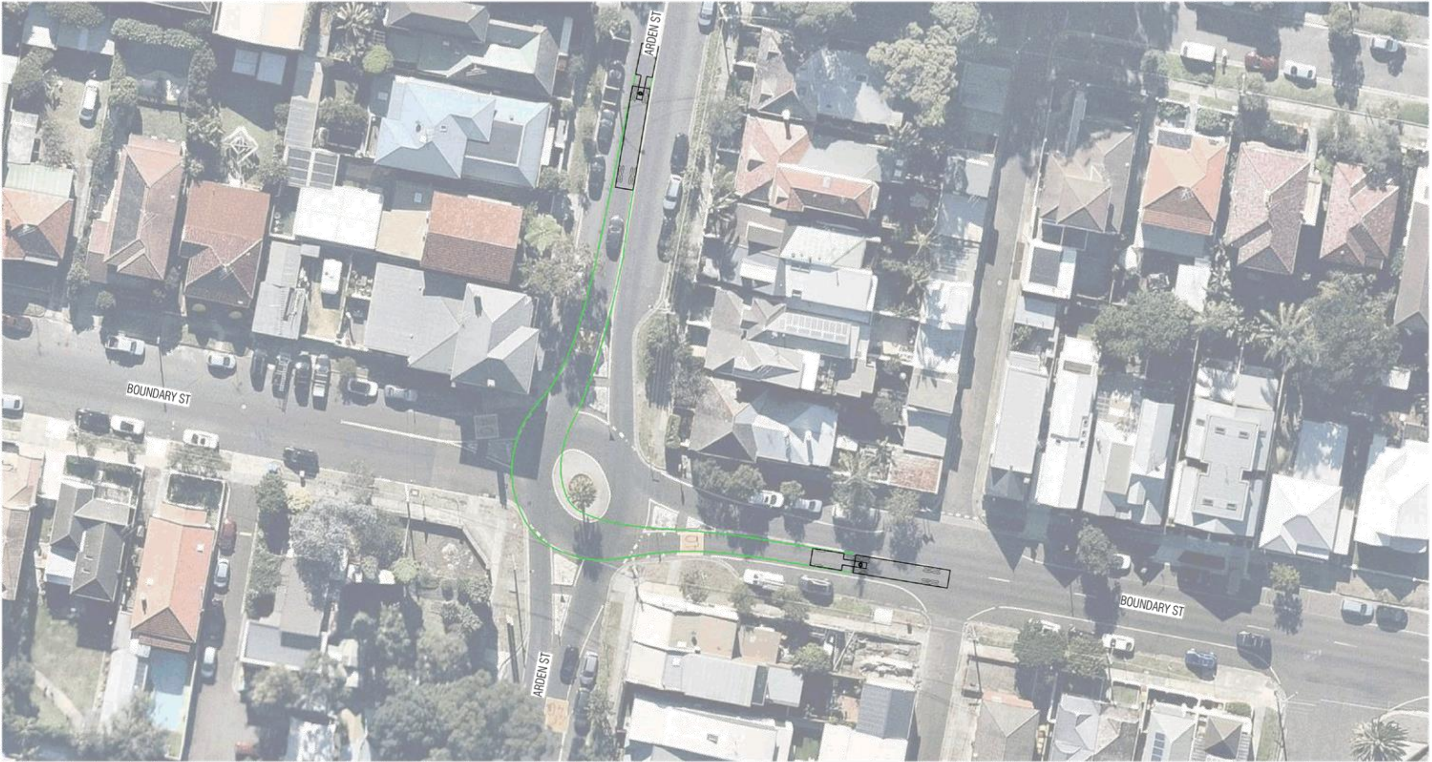
Boundary St Turning Right into Arden St Swept Path
