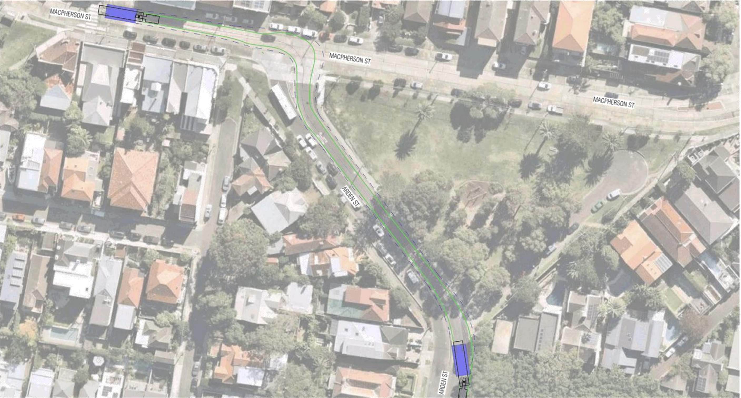
MacPherson St Turning Right into Arden St Swept Path
