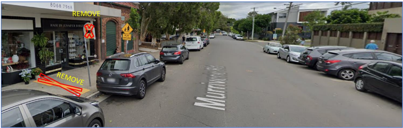
Figure 14. Proposal removal of J-stem and DDA tactiles at bus stop ID 202681.
