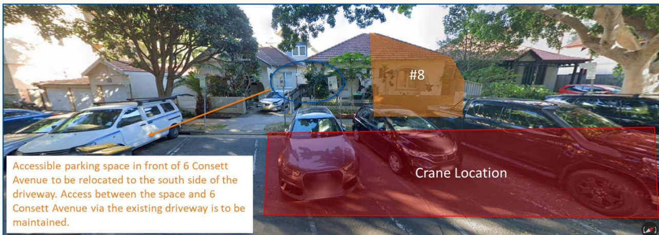
Figure 2. Crane standing location.
