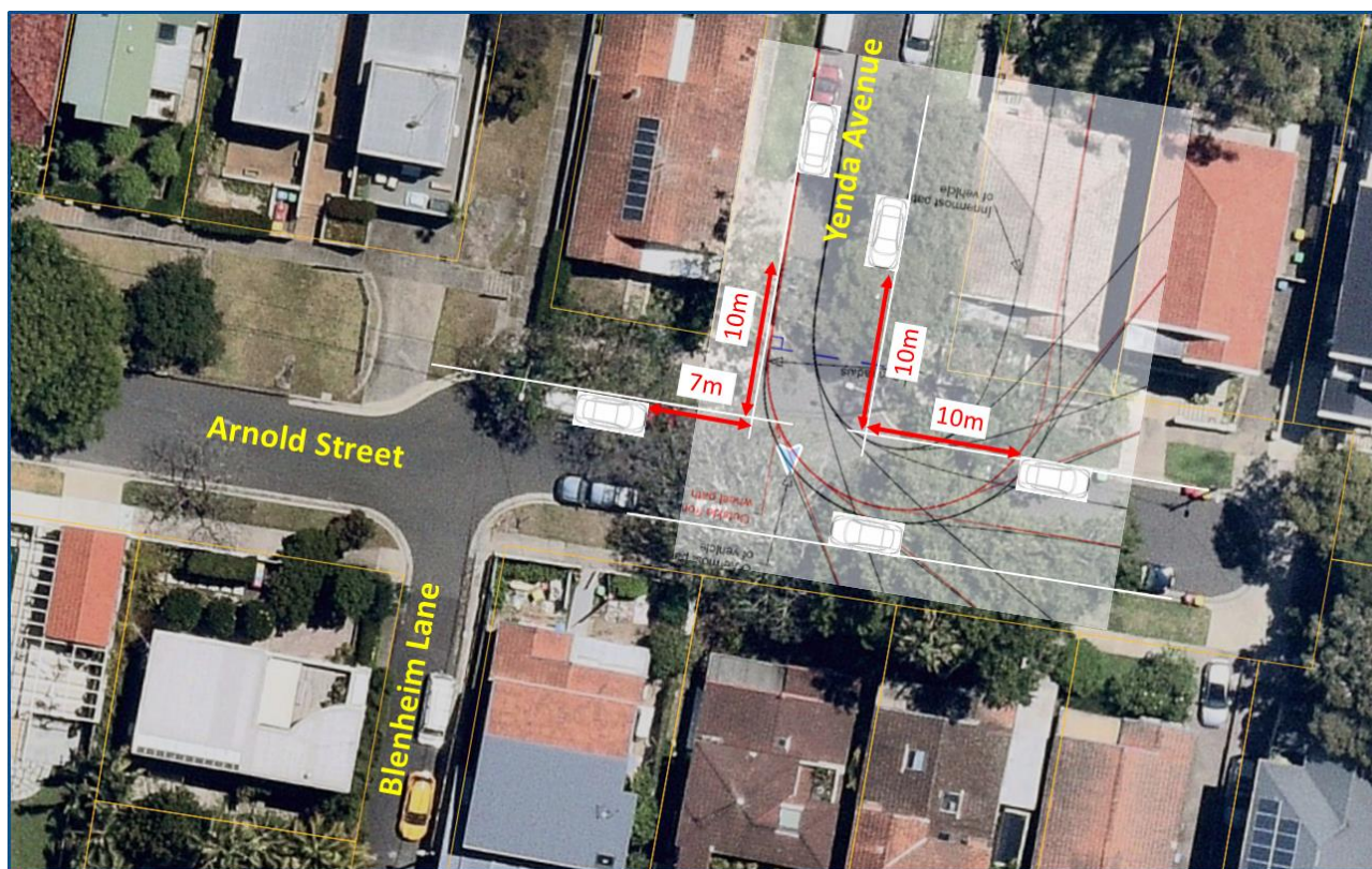
Figure 5. Swept path of medium rigid vehicle reversing from east end of Arnold Street into Yenda Avenue.
