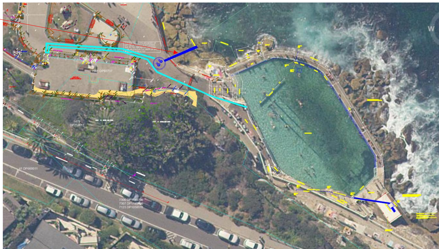
Figure 4: Option 3 – New wet well in the amenities forecourt and a new pump intake located close to the existing sea wall
