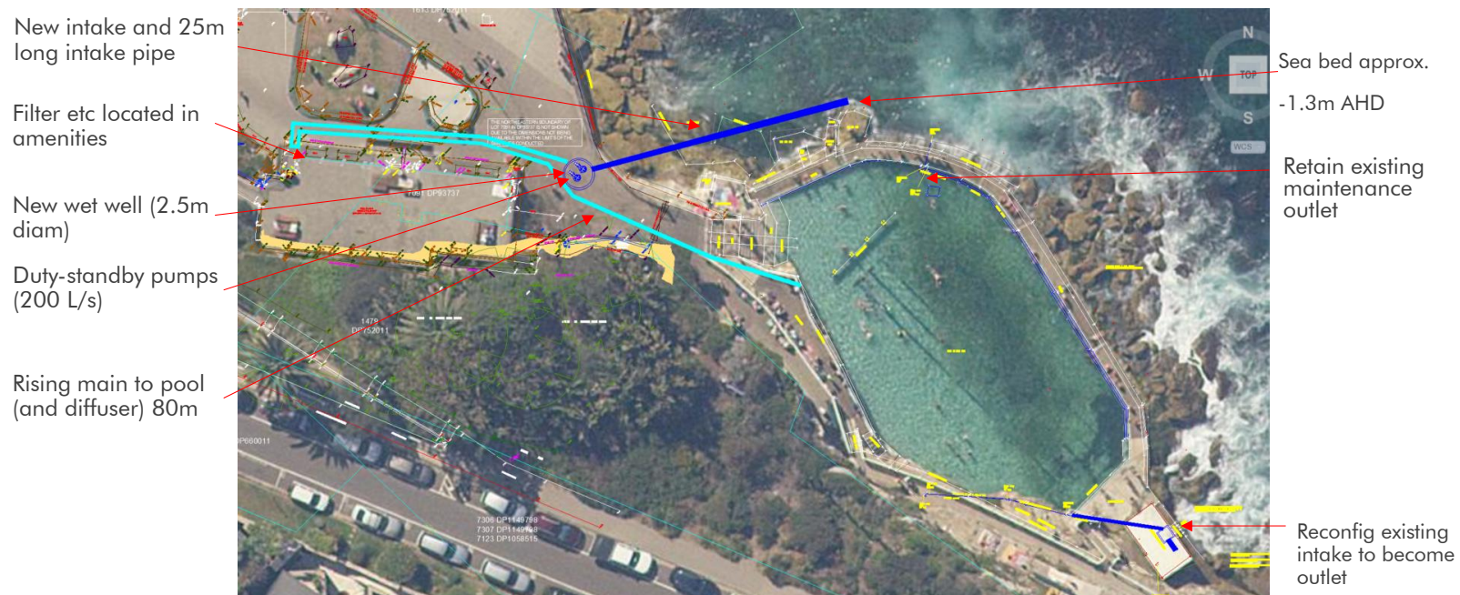
Figure 3: Option 2 – New wet well in the amenities forecourt and a new pump intake located in deeper water close to existing steps from pool to ocean
