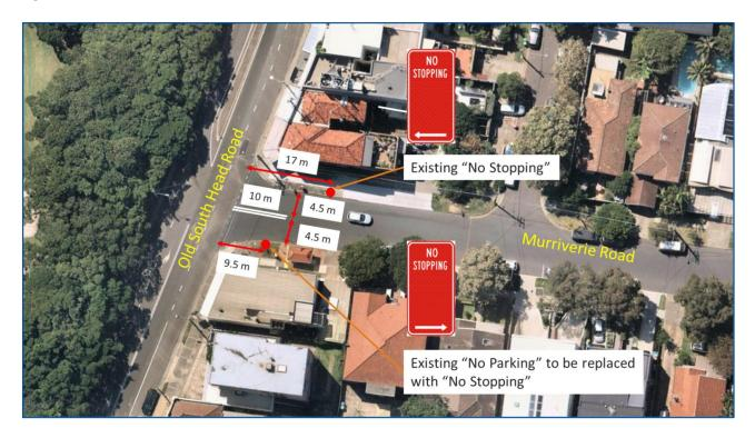
Figure 2. Proposed double centre line and "No Stopping" zone.
