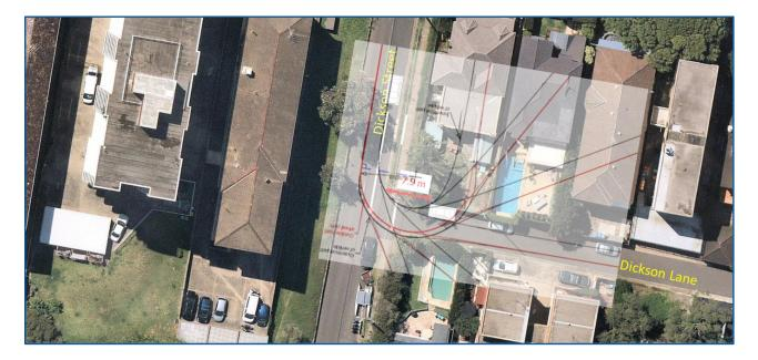
Figure 4. Swept path for Council waste vehicle turning left from Dickson Street onto Dickson Lane.
