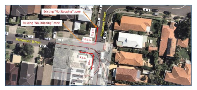
Figure 4. Swept path analysis diagram.
