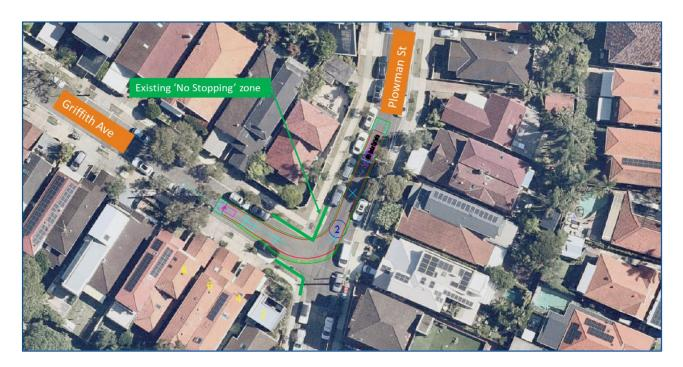
Figure 4. Swept path for medium rigid vehicle.
