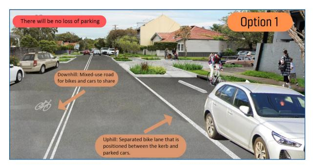
Figure 2. Uphill cycleway positioned between the kerb and parked cars.
