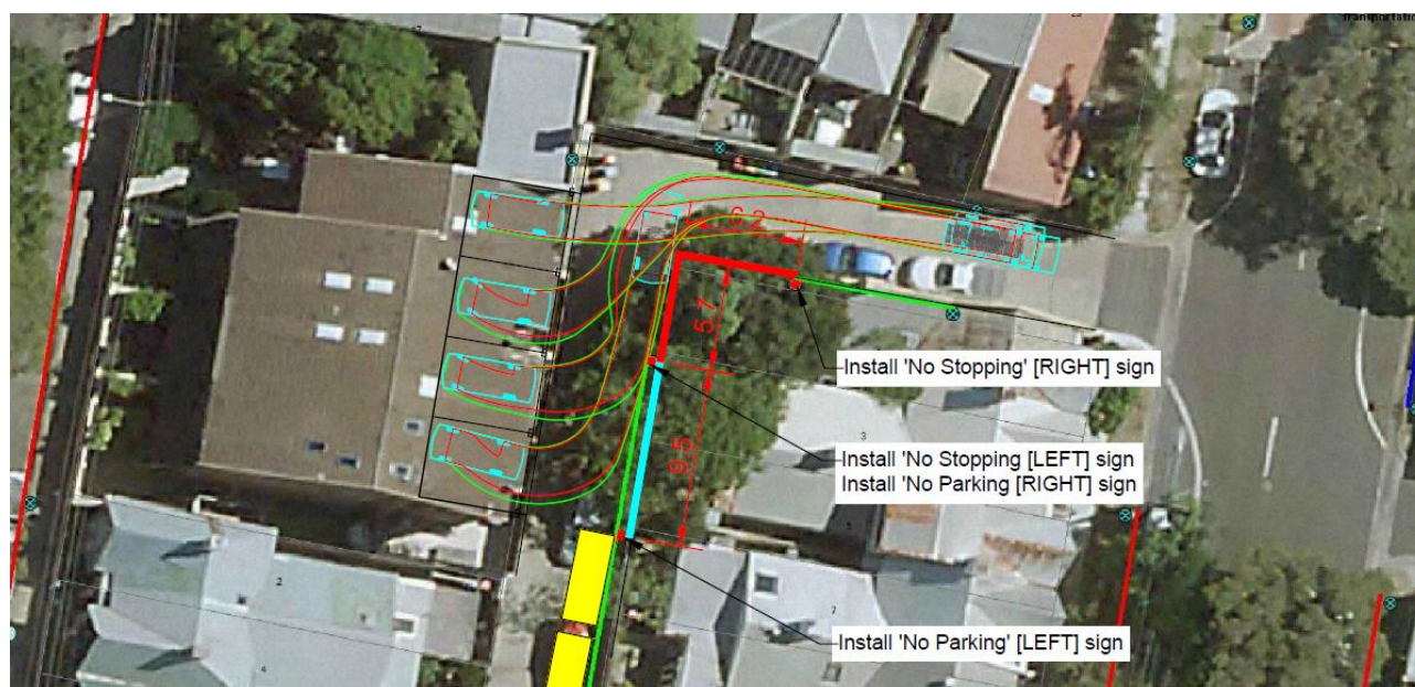
Figure 5. Swept wheel path of B85 vehicle – Proposed No Parking and No Stopping zone.
