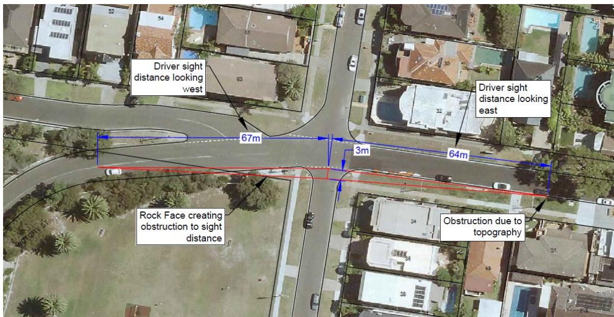
Figure 5. Existing sight distances in Portland Street northbound measured at a setback of 3m from the intersection and at a height of 1.05 m as per the Australian Standards.
