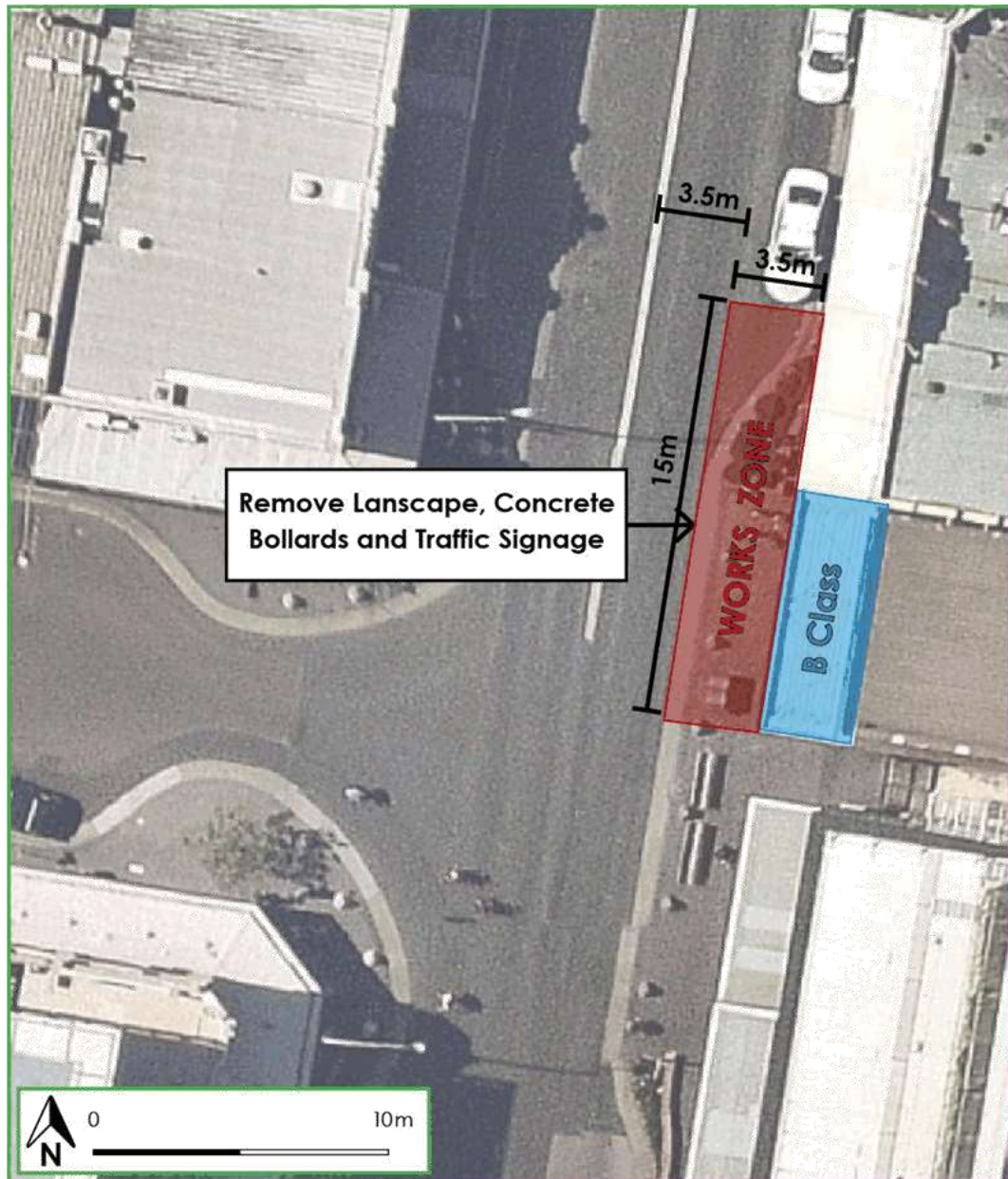
Figure 6: Proposed Work Zone and B-Class Hoarding
