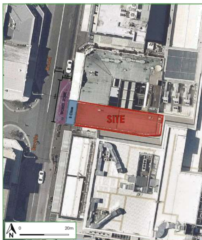
Figure 5: Proposed Works Zone and Class-B Hoarding during Construction Stages
