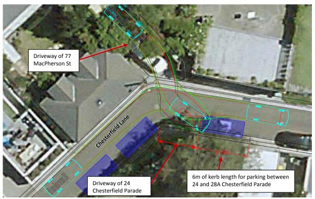
Figure 2: Shows the swept wheel path of a standard B85 vehicle entering and exiting the garage of 77 MacPherson Street
