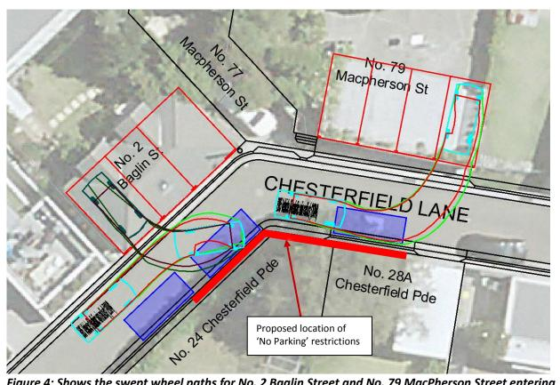
Figure 4: Shows the swept wheel paths for No. 2 Baglin Street and No. 79 MacPherson Street entering their respective garages from Chesterfield Lane and the proposed 'No Parking' zone
