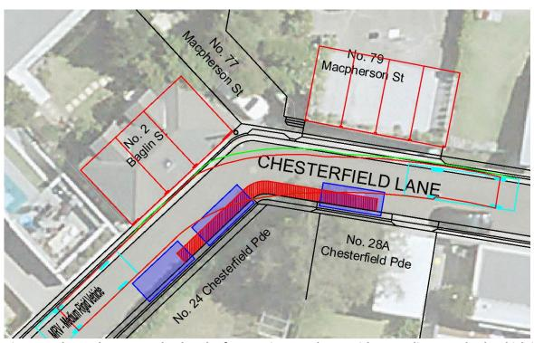
Figure 5: shows the swept wheel path of a MRV in accordance with Australian Standards which is similar in size to Council's garbage trucks
