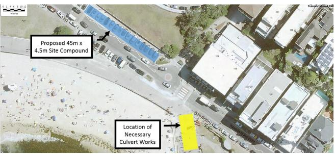
Figure 1. Proposed site compound and location of Council culvert works.
