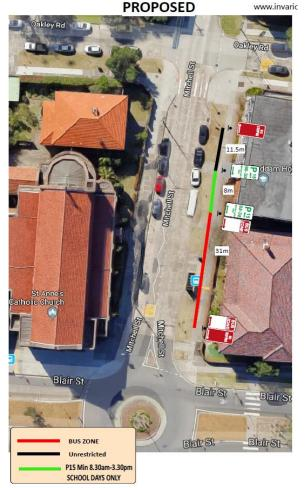
Figure 2: Mitchell Street – Existing and Proposed Parking arrangement.
