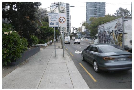
Photo 3: Poorly placed double post sign creates path 'squeeze point' adjacent to 83 Old South Head Road.
