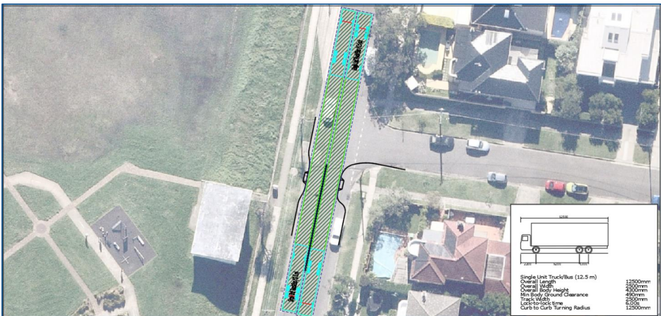
Figure 7. 12.5m bus swept paths with the proposed kerb buildout.
