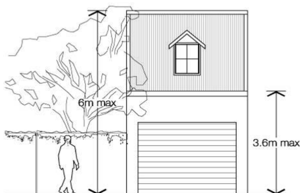
Figure 13 Maximum overall and external wall height for laneway development
