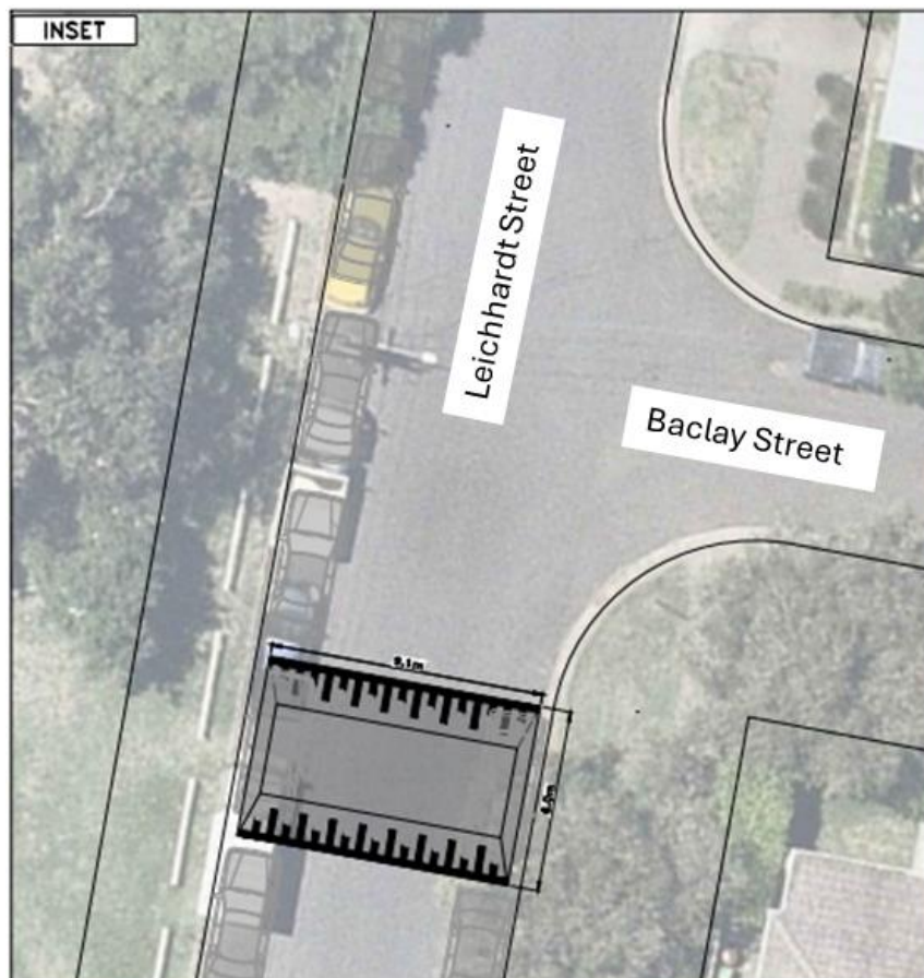
Figure 9. Recommended traffic calming device – Speed hump.
