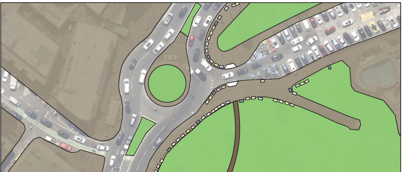
Figure 3. Traffic modelling Option B Scenario – Closed a portion of the roundabout.
