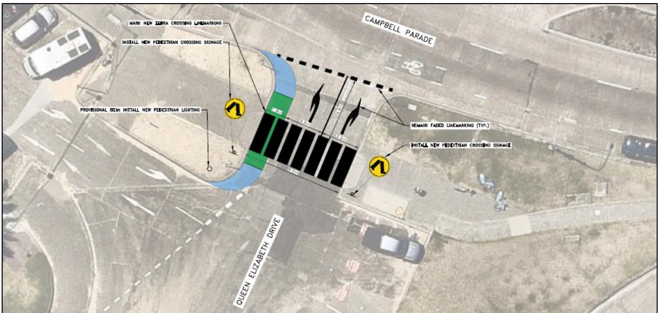
Figure 6. QED exit concept design crossing.
