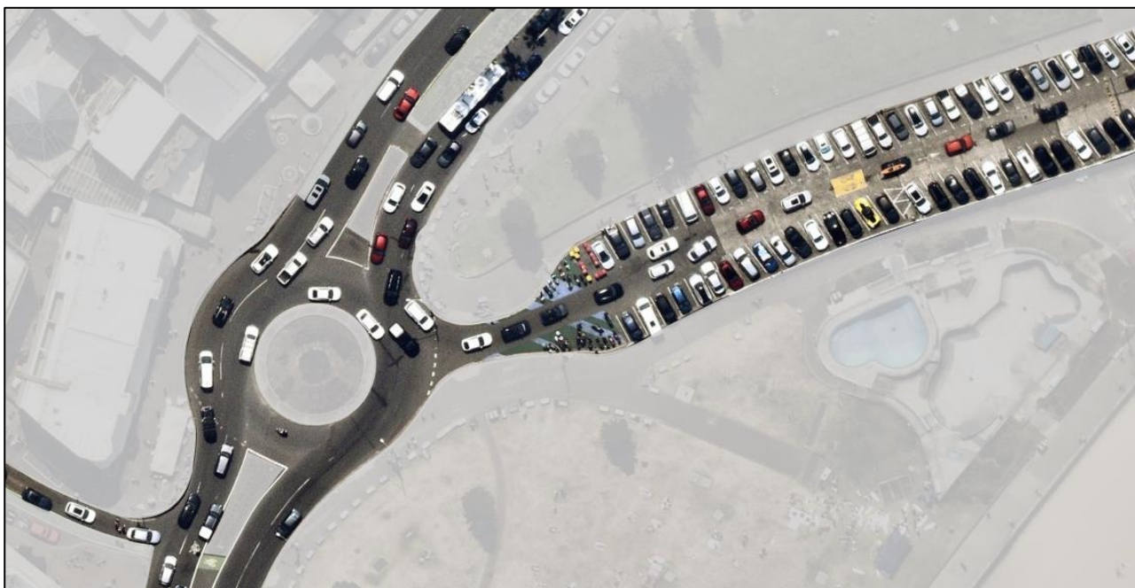
Figure 4. Vehicles queueing inside QED and propagating back towards the roundabout.
