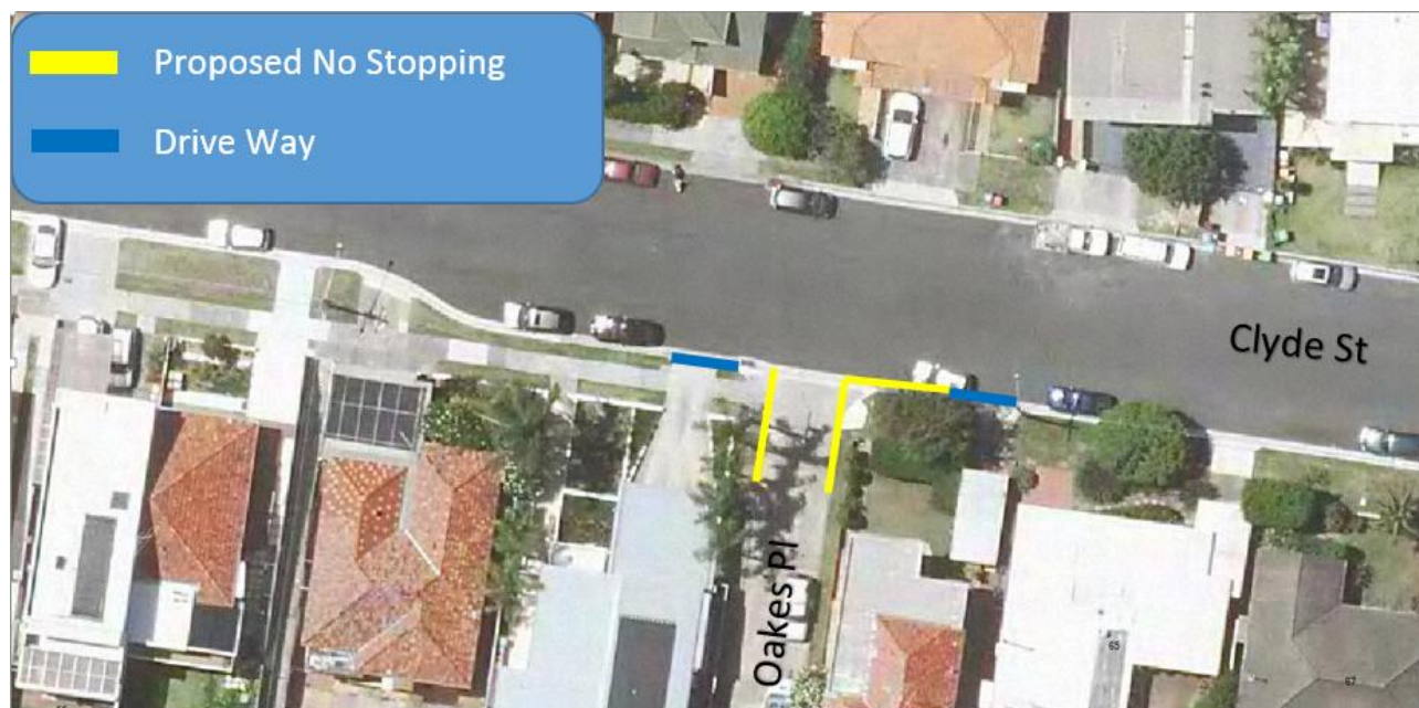
Figure 2.2 Proposed restrictions at intersection of Clyde Street and Oakes Place, North Bondi
