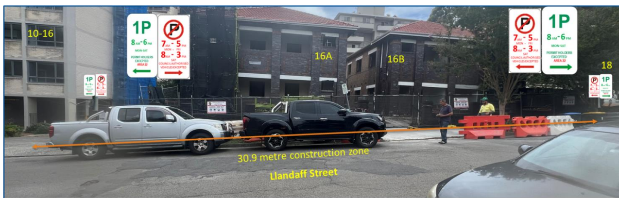
Figure 2. Location to install construction zone signs.
