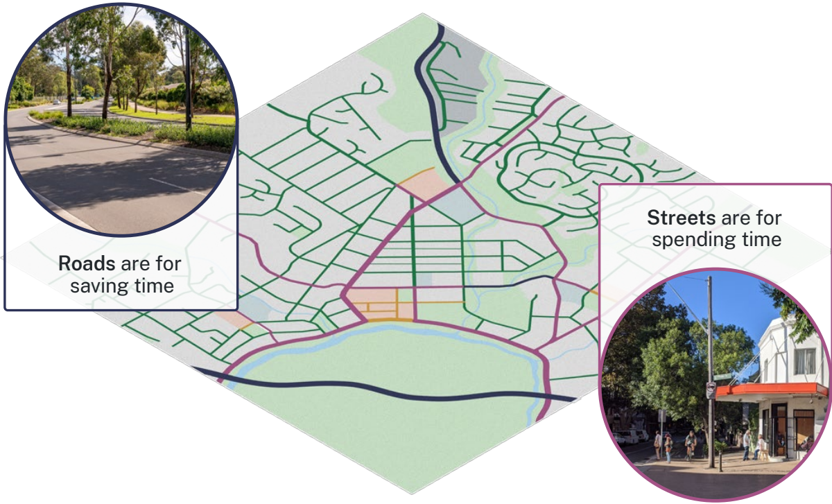
Figure 2. The functional difference between roads and streets
